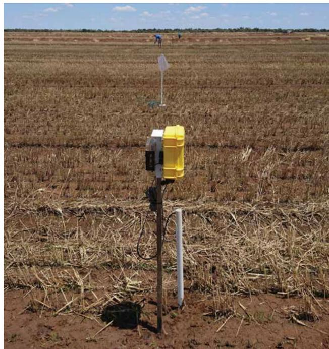
**A multi-level capacitance probe sensor installed at rice sowing time. The installation of the sensor with half above and half below the ground allows a full characterisation of the rice growing environment (soil-water-ambient) from a single robust probe.**
