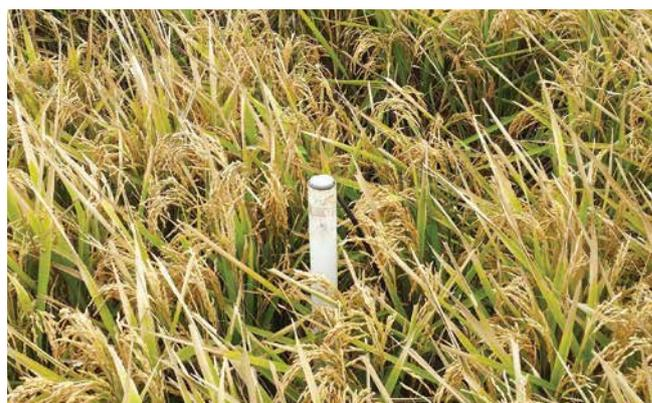
**The same multi-level capacitance probe sensor as pictured above, just prior to rice harvest.**
