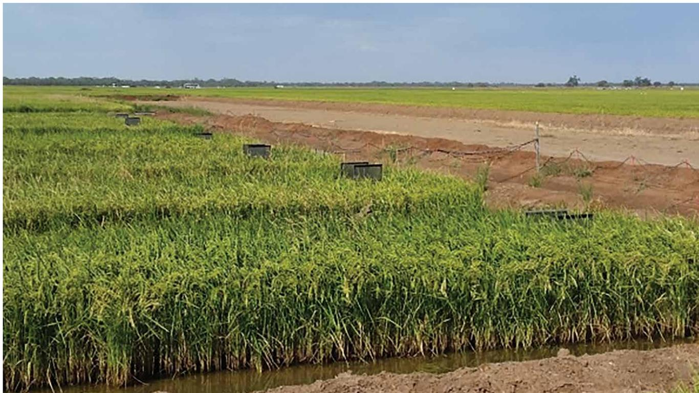
**Autochambers used to quantify methane and nitrous oxide emissions in the 2015–16 season.**
